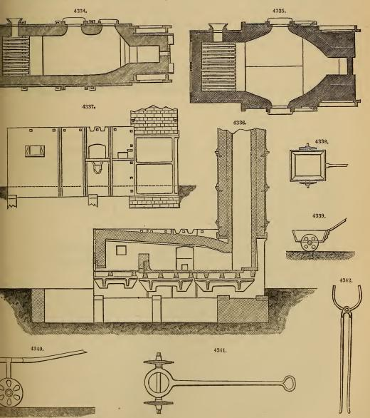
Cyfarthfa Iron-works; Figs. 4335 to 4337, plan, section, and side elevation of a common double puddling furnace; Figs. 4338, 4339, tub for einder; Figs. 4340, 4341, carriage for conveying
